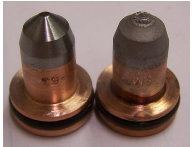
Figure 6 Comparison of New vs. Used Electrode
