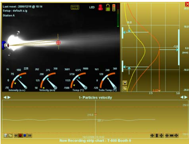
Figure 3 Plume Profile of Another Powder (orange line) with Target Powder (yellow line)-Booth C. Note 600°C difference in temperature
