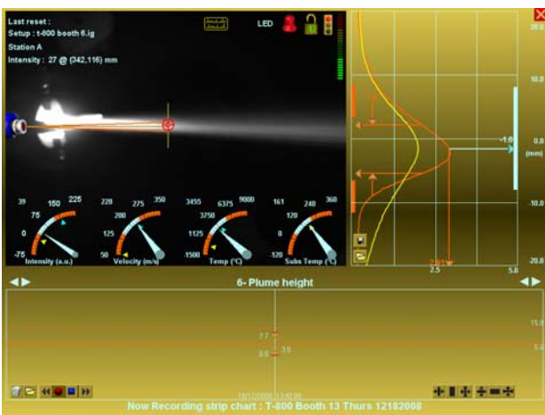
Figure 4 Plume Profile of Target Powder(orange line) in Booth D compared with same Target Powder (yellow line) in Booth C. Note 400°C difference in temperature and increased velocity
