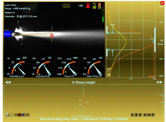
Figure 5 Plume Profile of New Powder(orange line) in Booth D compared with original Target Powder (yellow line)-Booth C. Note 1000°C difference in temperature and increased velocity.
