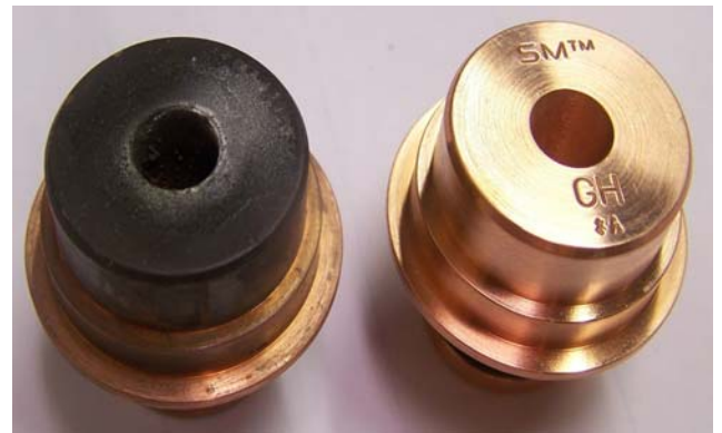
Figure 7. Comparison of New vs. Used Nozzle
