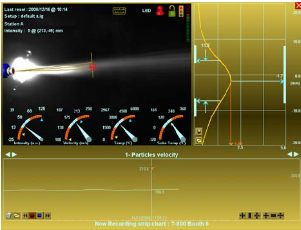
Figure 2 Plume Profile of Target Powder with Acceptable Results (yellow line)-Booth C
